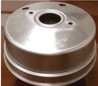
A stamper was trying to reduce splitting and cracking while also improving the cleanability of 5XXX series aluminum housing parts using a next-gen, HSE-focused soluble oil.
