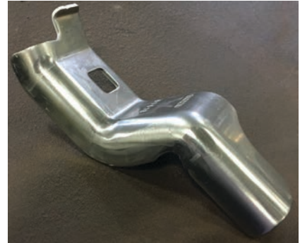
A CP soluble oil used on a 0.100-in.-thick 5XXX series aluminum automotive part created welding problems downstream.
