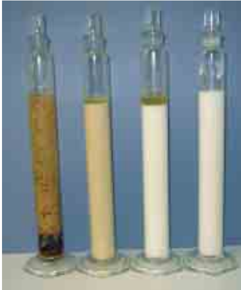
Fig. 2—The Stability Test finds use when using a water-based lubricant. While many water-based lubricants will initially mix readily with water, the long-term stability of the water-based mixture is of great importance. Should the lubricant separate or split, the lubricant that reaches the workpiece could be severely diluted.
