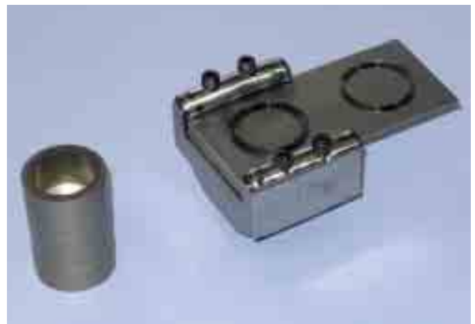
Fig. 3—The Twist Compression Test measures friction and evaluates adhesion in metalforming. It uses contact pressures set to match the process. This test measures the transmitted torque between a rotating annular cylinder and a lubricated flat-sheet specimen. Tooling and stock material can be mirrored to the exact application to find the best-suited materials.
