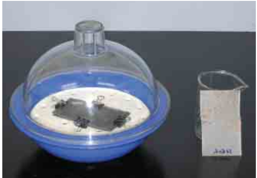
Fig. 1—The Stack-Stain Test determines lubricant staining if parts or material stack flat upon one another, trapping lubricant under a load. This is a good test if shops stamp and stack blanks, then store them for some time before final processing.
