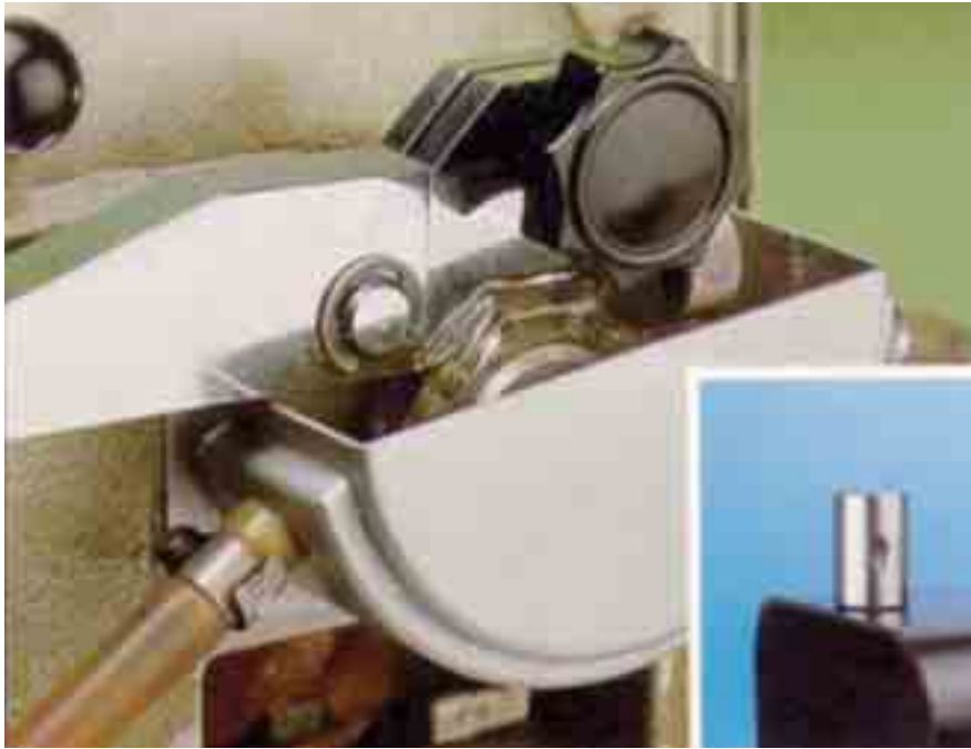
Fig. 4—The Reichert Test determines the load-carrying capacity of a lubricant. The test uses a weighted lever arm, with a wear pin, on a rotating race in a lubricant sump. The stamper then analyzes the pin and race for wear patterns and comparisons.
